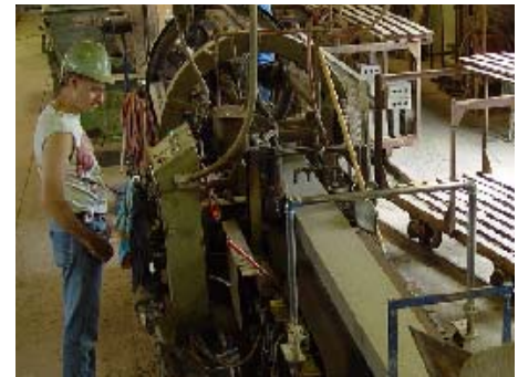
Reviewing a column of green brick as it departs the extruder
